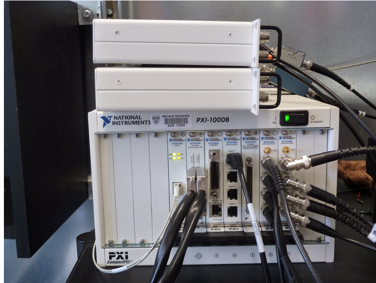
Figure C.1: National Instruments PXI chassis including digitizers, signal generators, and other instruments. The two PXI-4462 digitizer cards accept signals via direct BNC connection, while the PXI-6259 card, used for generating the lock-in reference signals, connects via the external breakout boxes sitting above the PXI chassis.
